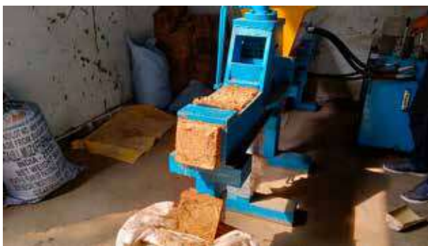
Processing of indigenous cow urine treated paddy straw complete fodder blocks
